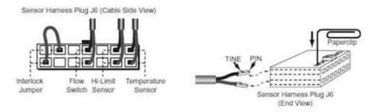
To remove a sensor or flow switch wire from the sensor harness connector J6, insert the end of a paper clip or similar device into the slot corresponding with the wire to be removed. This will depress the pin tine, allowing the wire to be pulled from the harness connector.
