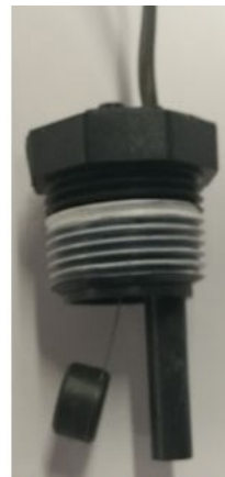
Flow Switch Open Disc Does Not Touch Post
