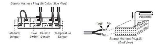
To remove a sensor or flow switch wire from the sensor harness connector J6, insert the end of a paper clip or similar device into the slot corresponding with the wire to be removed. This will depress the pin tine, allowing the wire to be pulled from the harness connector.
